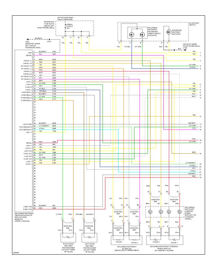
Fig. 54: Supplemental Restraints Circuit (1 of 2)
