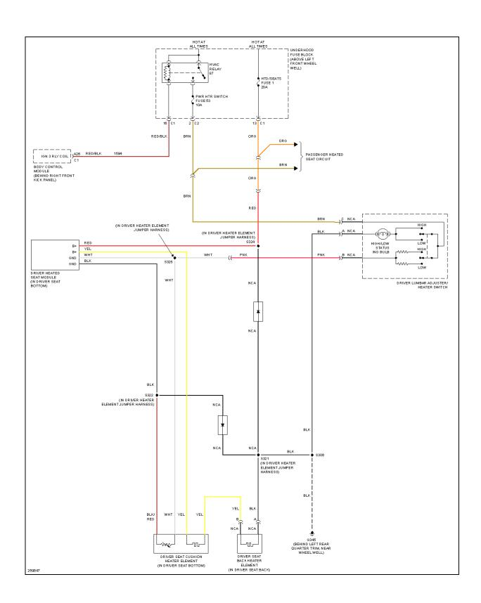
Fig. 38: Driver Heated Seat Circuit
