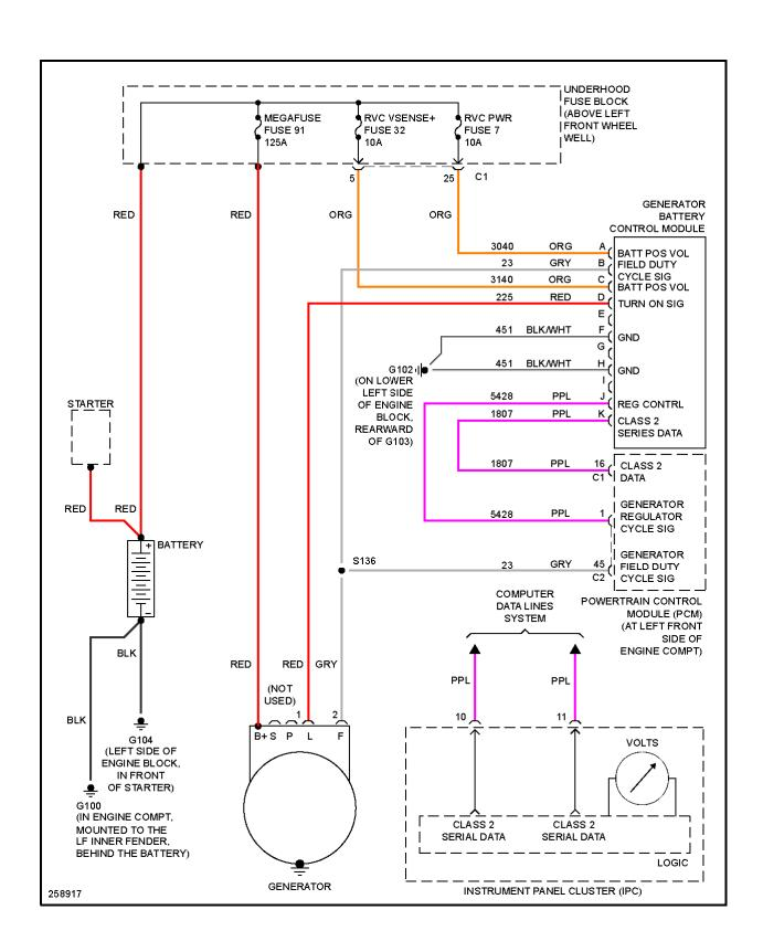
Fig. 51: Charging Circuit
