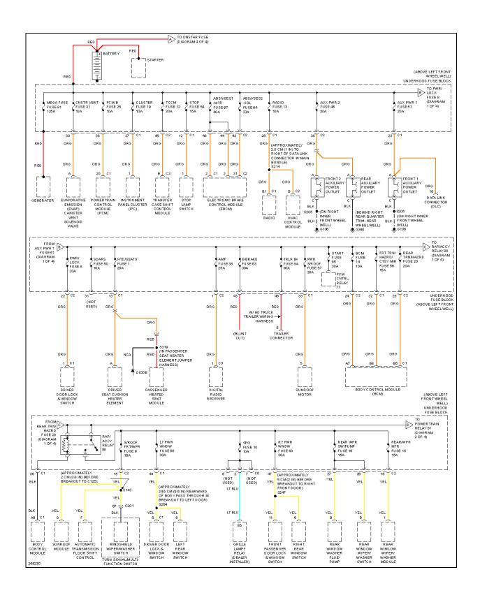
Fig. 31: Power Distribution Circuit (1 of 4)
