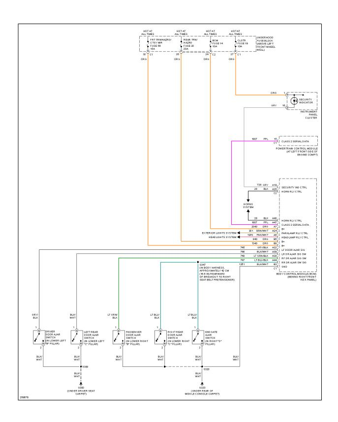
Fig. 6: Forced Entry Circuit
