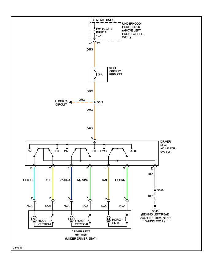
Fig. 39: Driver Power Seat Circuit
