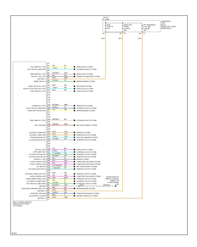
Fig. 8: Body Control Modules Circuit (1 of 2)
