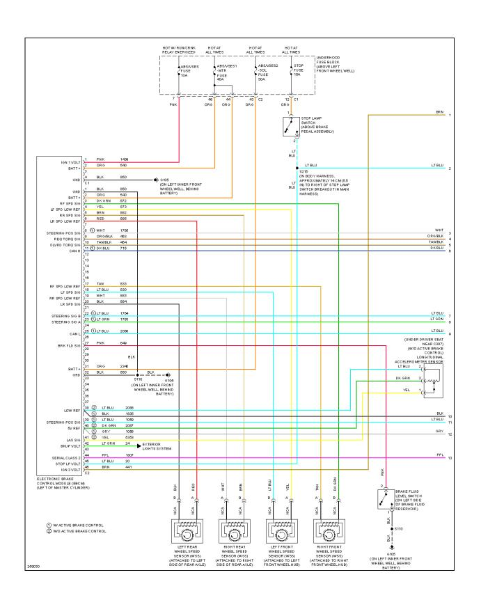
Fig. 4: Anti-lock Brakes Circuit (1 of 2)
