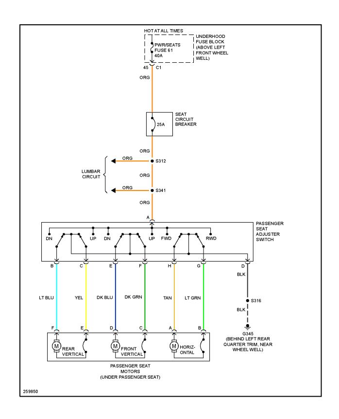
Fig. 41: Passenger Power Seat Circuit
