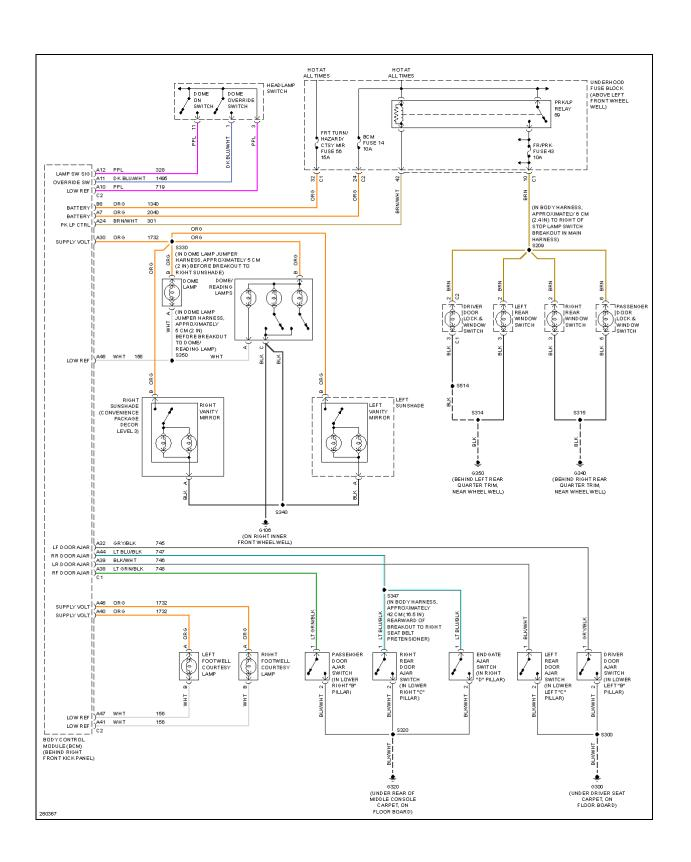
Fig. 28: Courtesy Lamps Circuit
