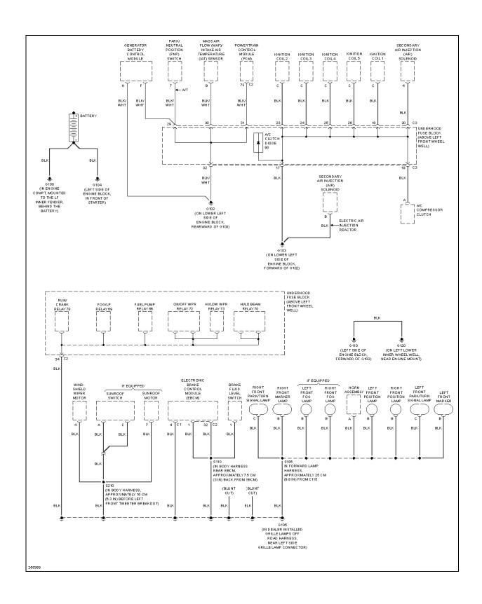
Fig. 22: Ground Distribution Circuit (1 of 3)
