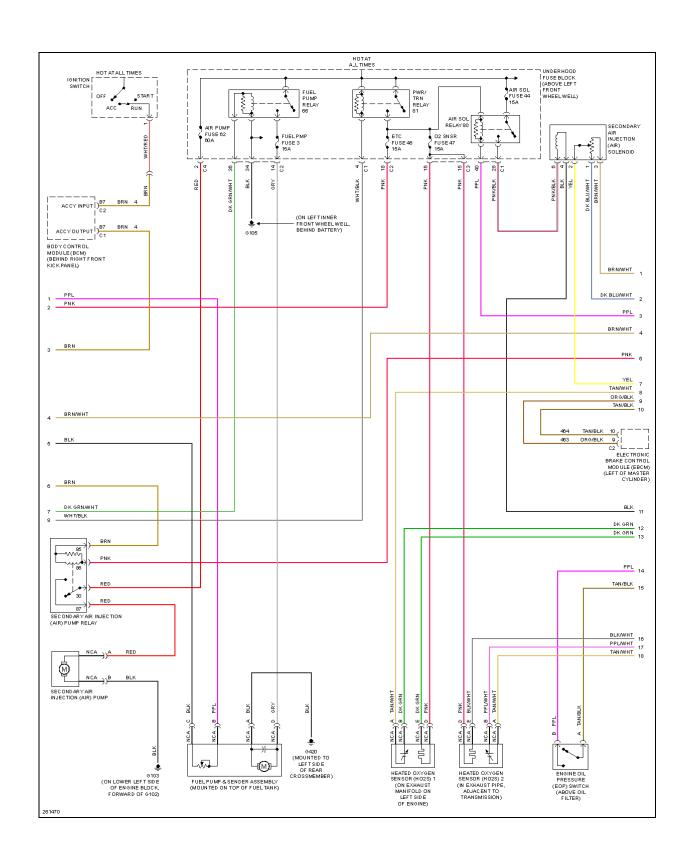
Fig. 14: 3.7L VIN E, Engine Performance Circuit (2 of 5)
