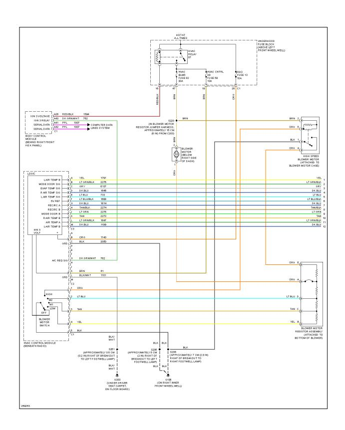
Fig. 2: Manual A/C Circuit (1 of 2)
