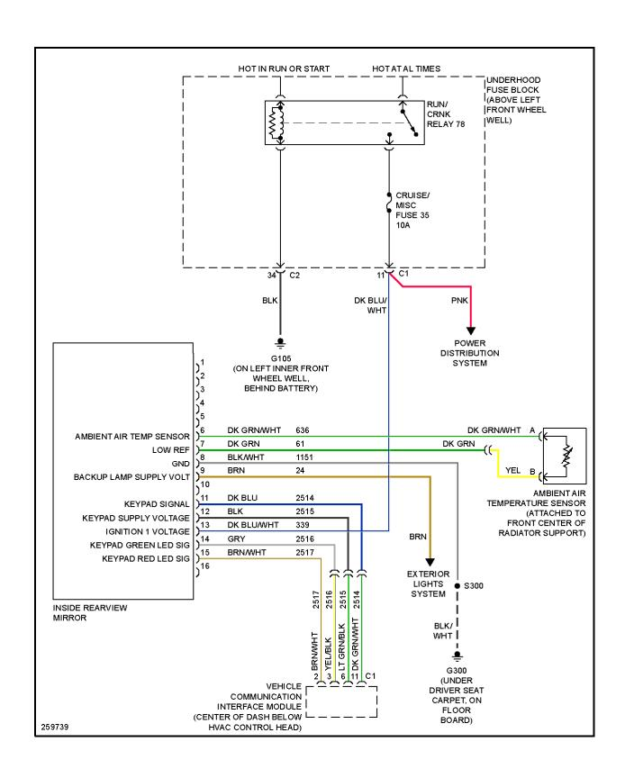
Fig. 36: Electrochromic Mirror Circuit
