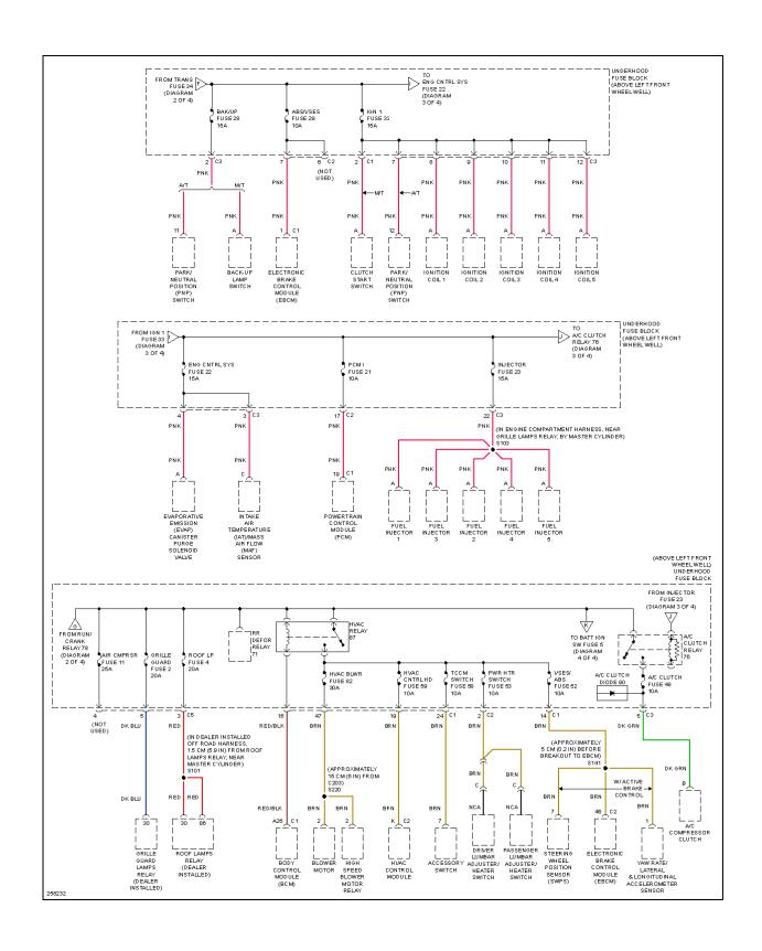
Fig. 33: Power Distribution Circuit (3 of 4)
