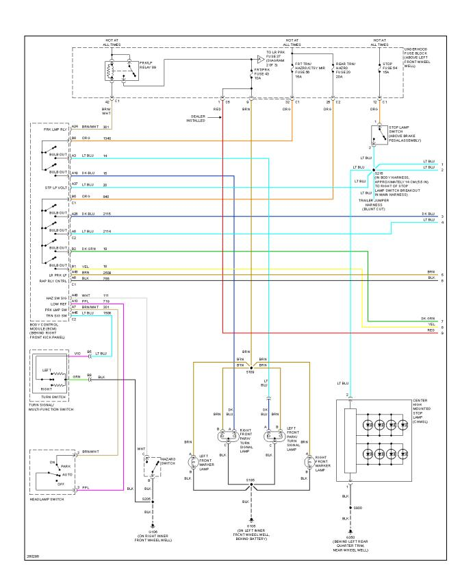
Fig. 19: Exterior Lamps Circuit (1 of 3)
