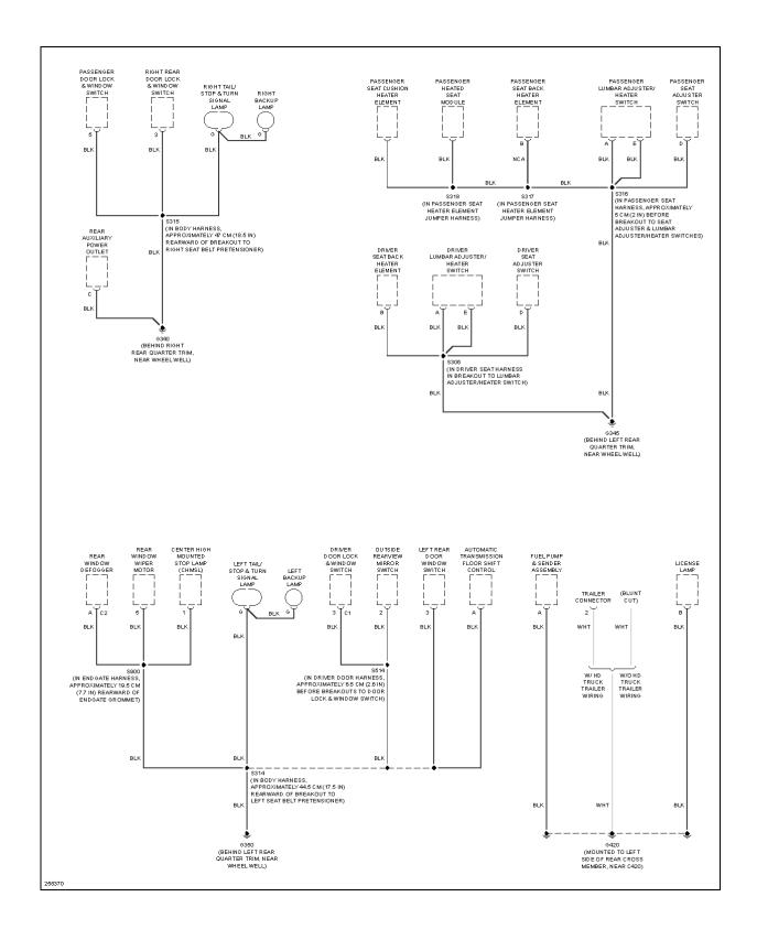
Fig. 23: Ground Distribution Circuit (2 of 3)
