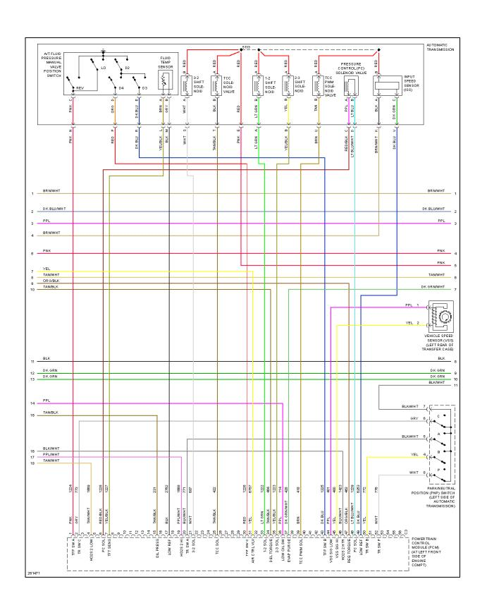
Fig. 15: 3.7L VIN E, Engine Performance Circuit (3 of 5)
