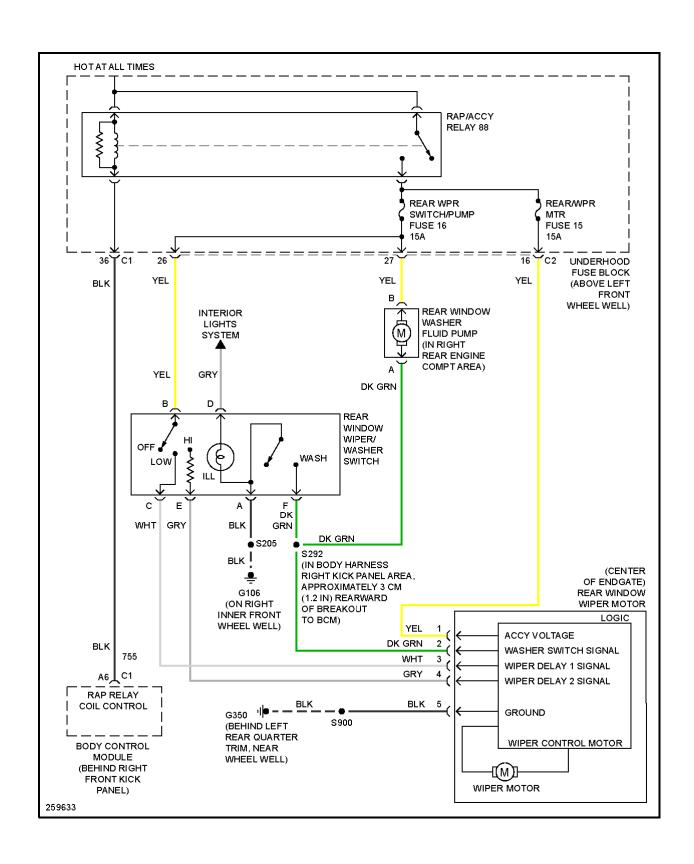
Fig. 60: Rear Wiper/Washer Circuit
