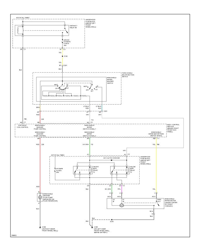
Fig. 59: Front Wiper/Washer Circuit
