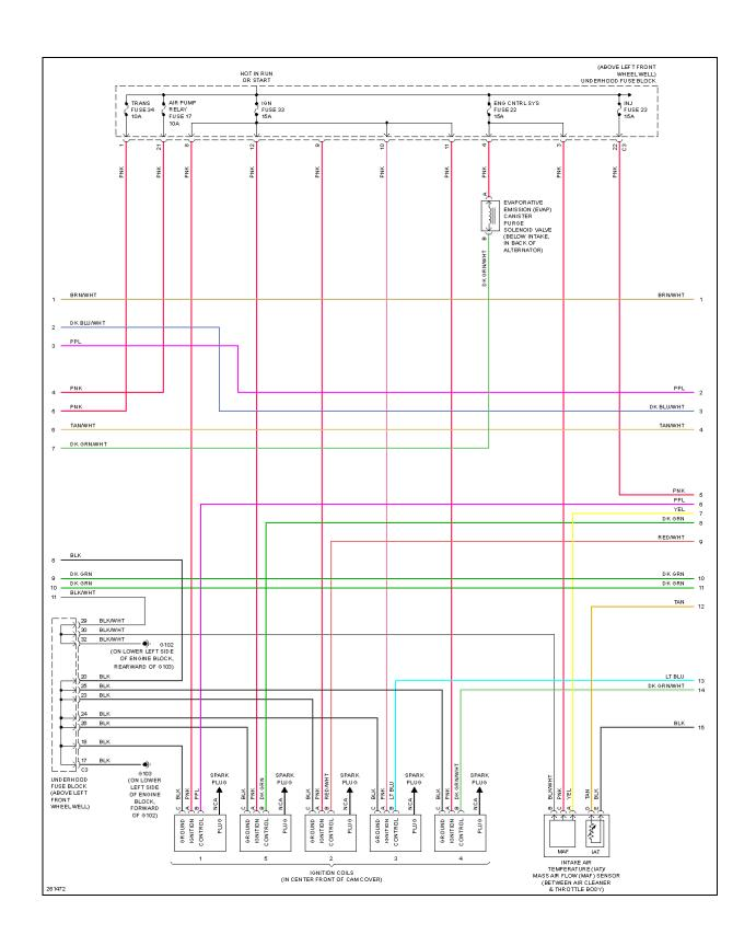
Fig. 16: 3.7L VIN E, Engine Performance Circuit (4 of 5)
