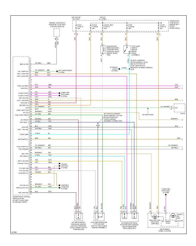
Fig. 13: 3.7L VIN E, Engine Performance Circuit (1 of 5)
