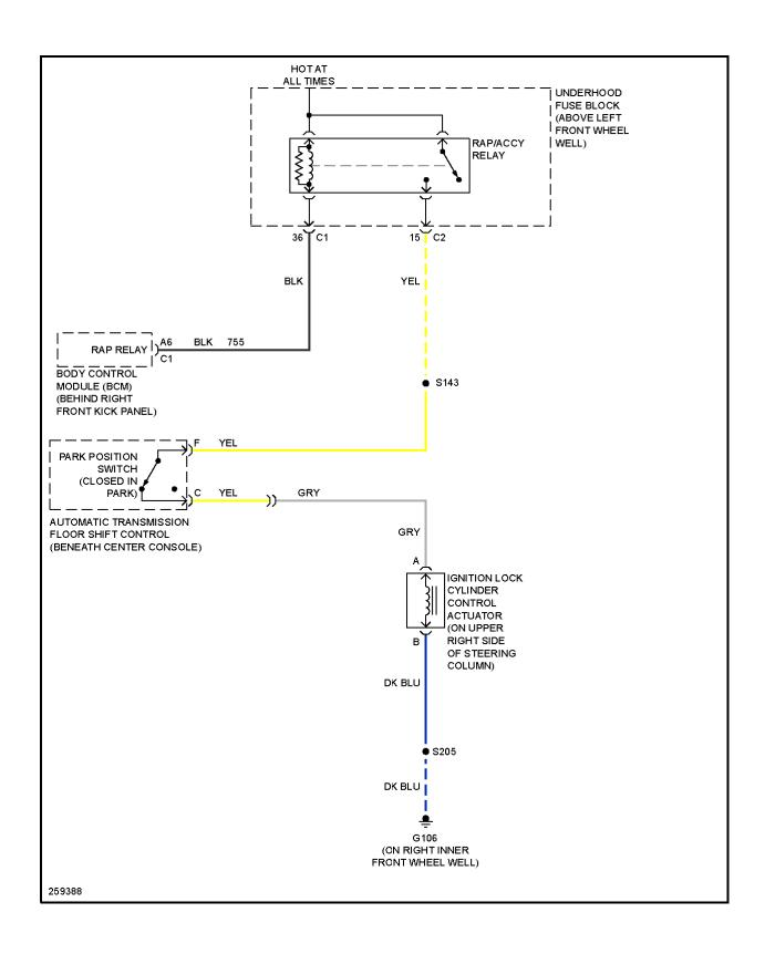
Fig. 49: Ignition Lock Solenoid Circuit
