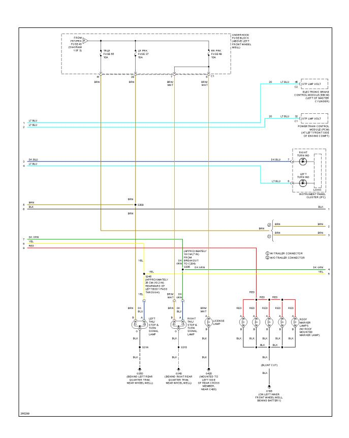
Fig. 20: Exterior Lamps Circuit (2 of 3)
