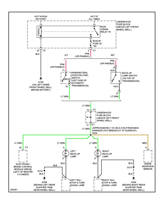
Fig. 18: Back-up Lamps Circuit
