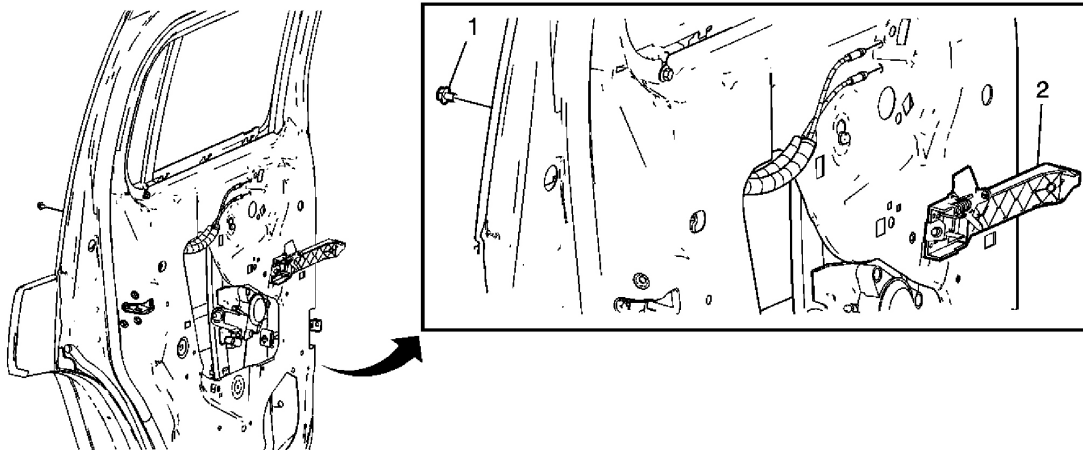
Fig. 22: Rear Side Door Outside Handle Housing Replacement Courtesy of GENERAL MOTORS CORP.
