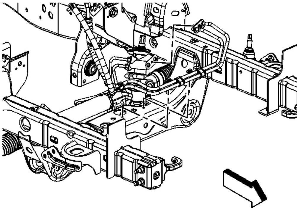
**Fig. 33: View Of Power Steering Hose Assembly**
