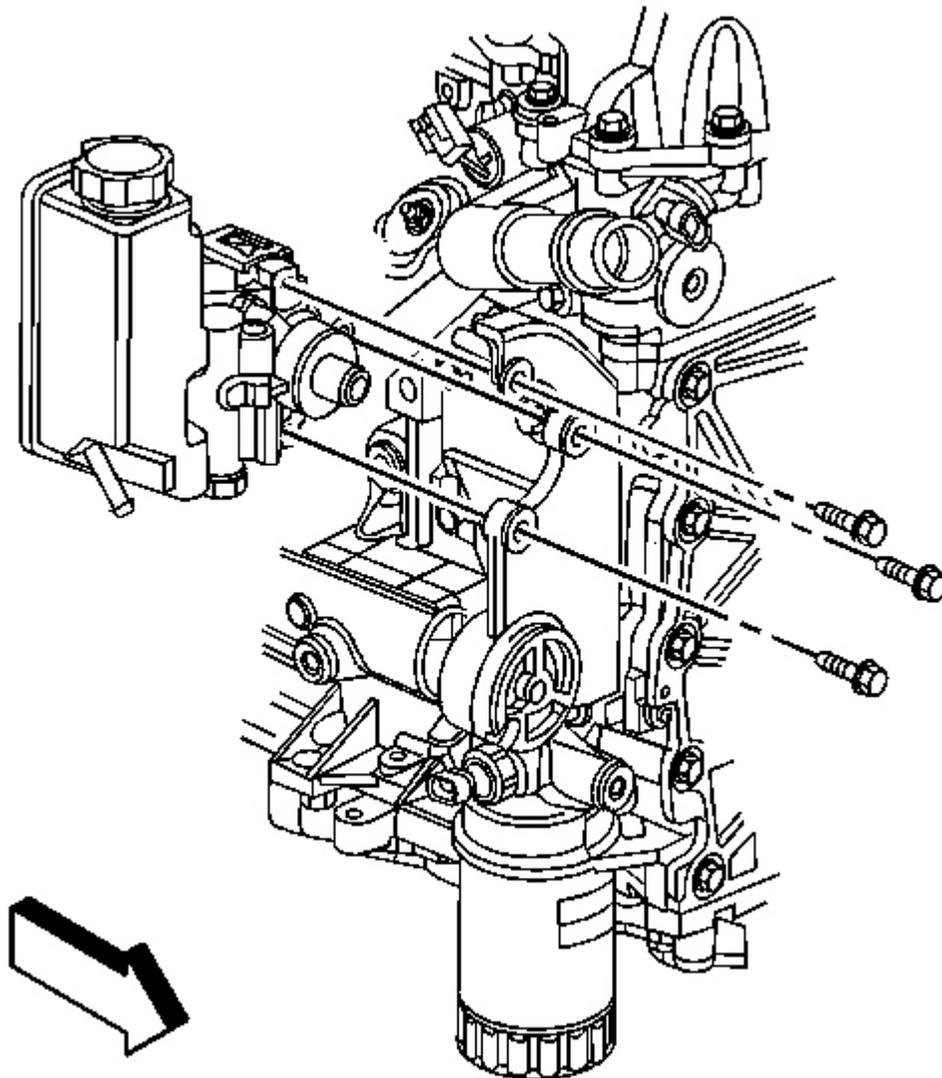
**Fig. 12: View Of Power Steering Pump & Mounting Bolts**
