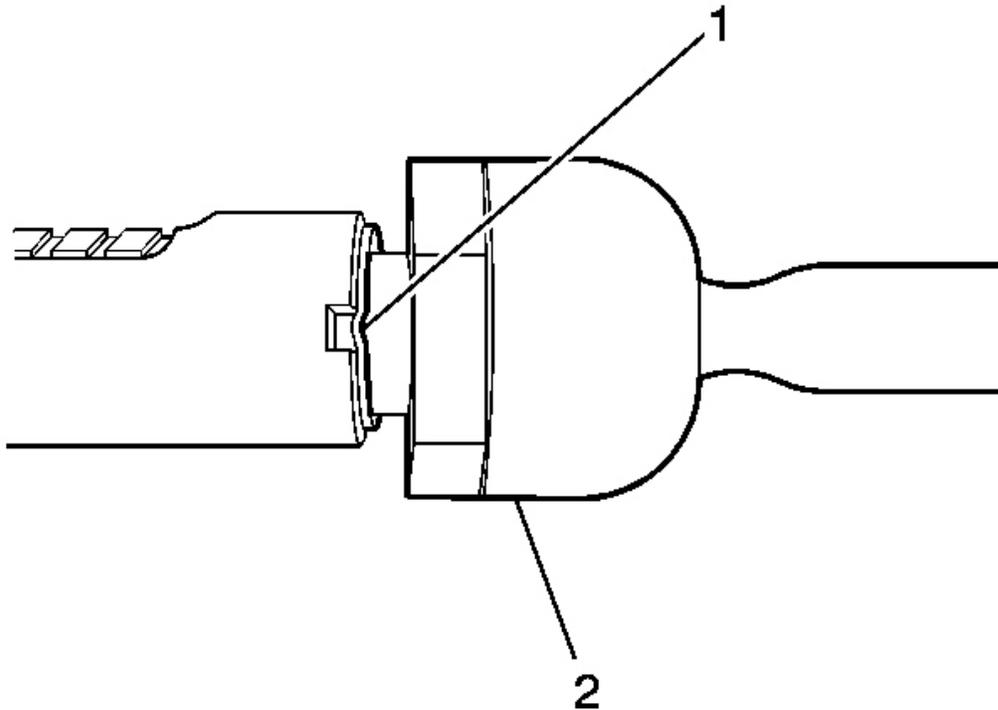
**Fig. 22: Identifying Inner Tie Rod Staking Location**
