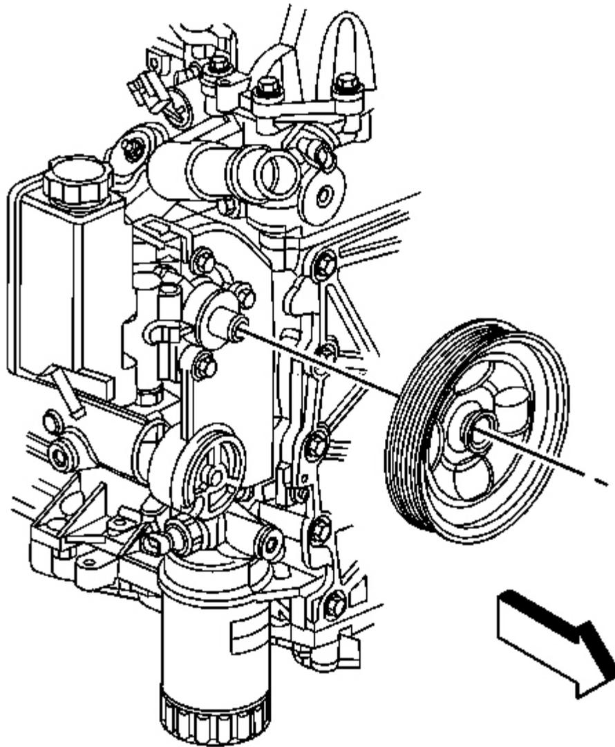
**Fig. 7: View Of Power Steering Pump Pulley**
