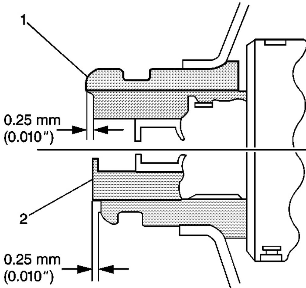
**Fig. 9: Checking Power Steering Pump Pulley Installed Depth**
