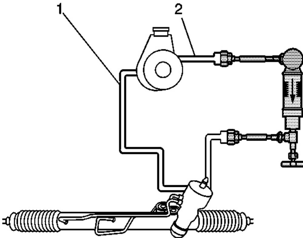
**Fig. 1: Testing Rack and Pinion System Pressures**
