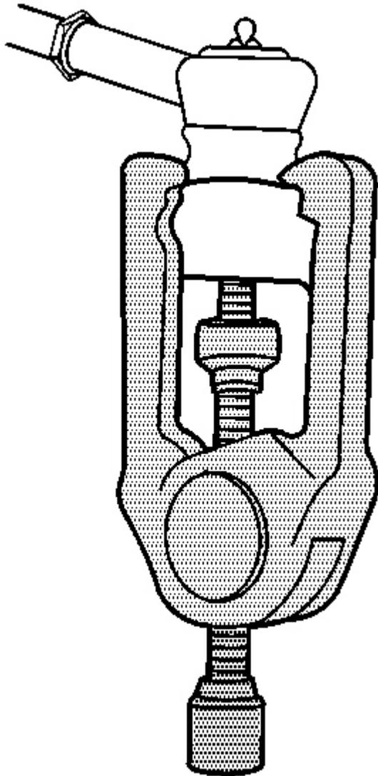
**Fig. 17: Removing Outer Tie Rod Assembly From Steering Knuckle**
