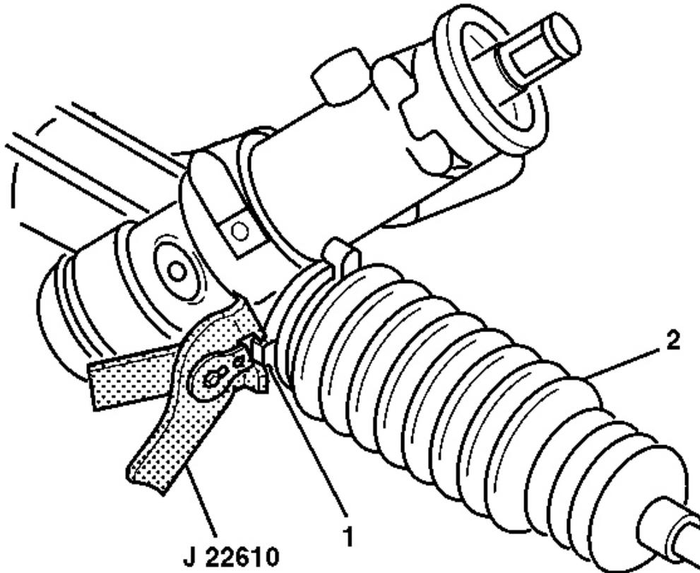
**Fig. 28: Using J 22610 To Install Boot Clamp**
