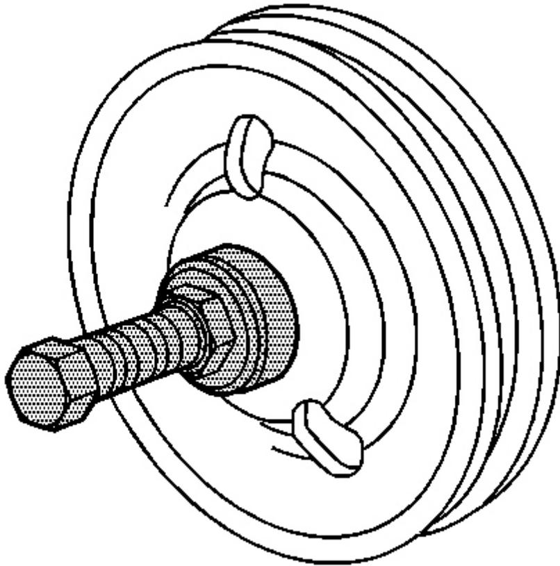
**Fig. 8: View Of Power Steering Pump Pulley Installer**
