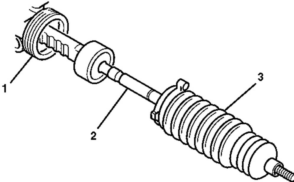
**Fig. 27: Rack & Pinion Gear Assembly, Boot & Inner Tie Rod Assembly**
