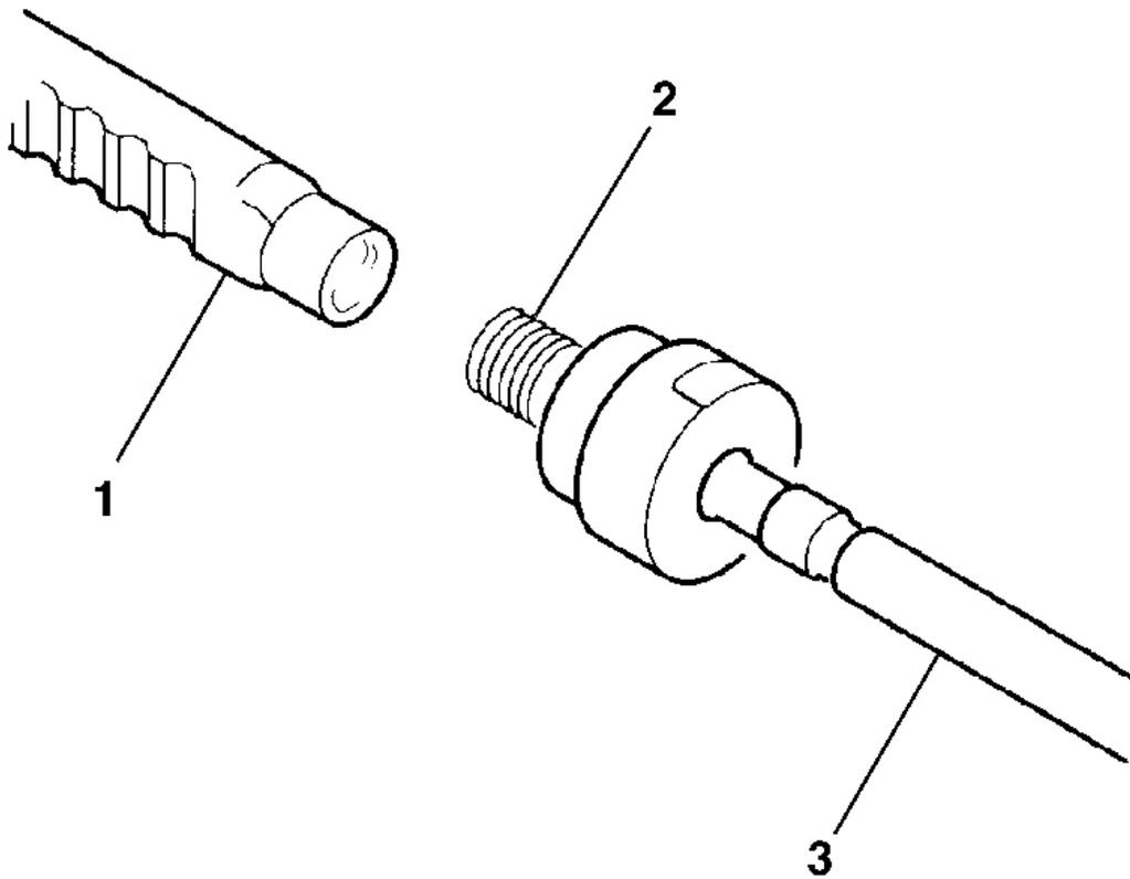
**Fig. 20: View Of Rack And Inner Tie Rod Threads**
