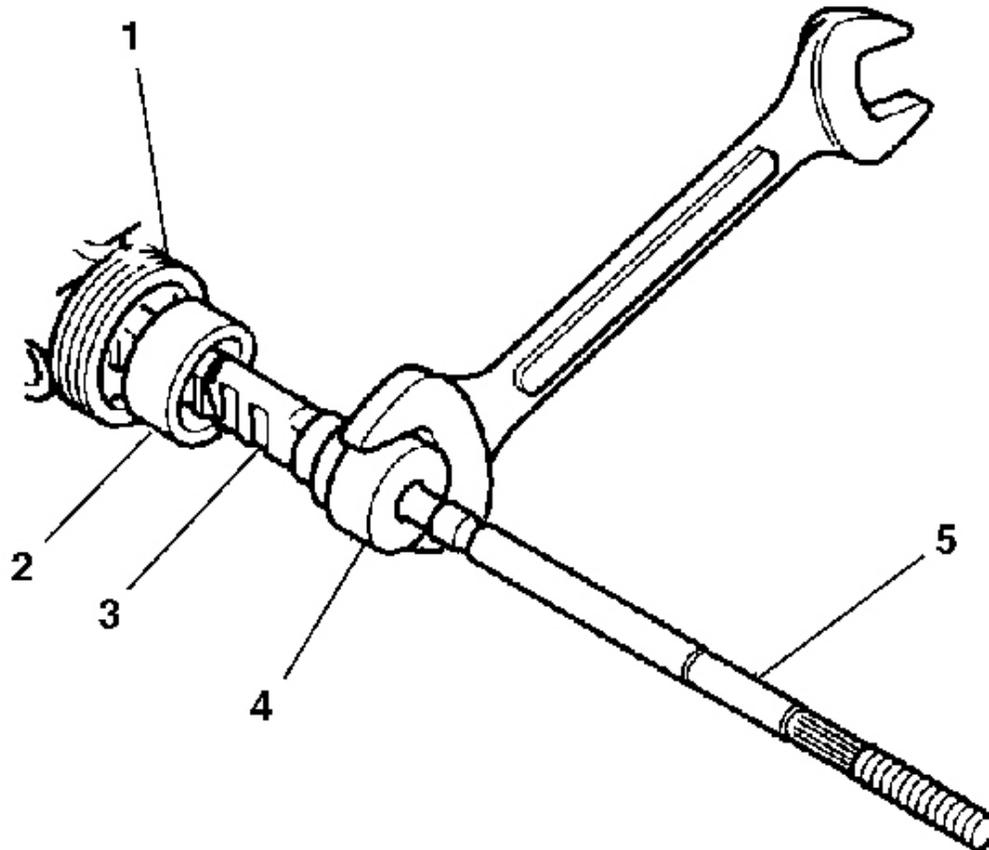
**Fig. 19: Removing The Shock Dampener From The Inner Tie Rod**
