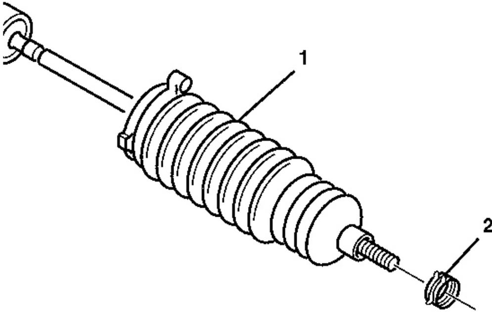
**Fig. 29: View Of Tie Rod End Clamp At Rack & Pinion Boot**
