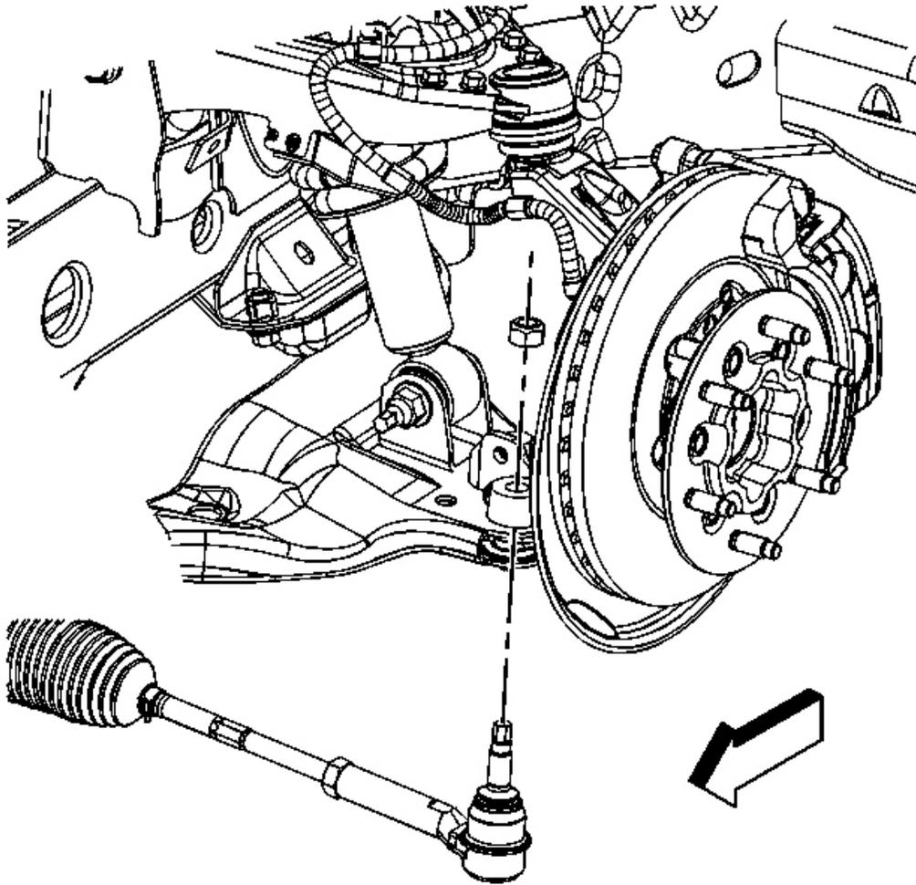
**Fig. 16: View Of Outer Tie Rod Retaining Nut**
