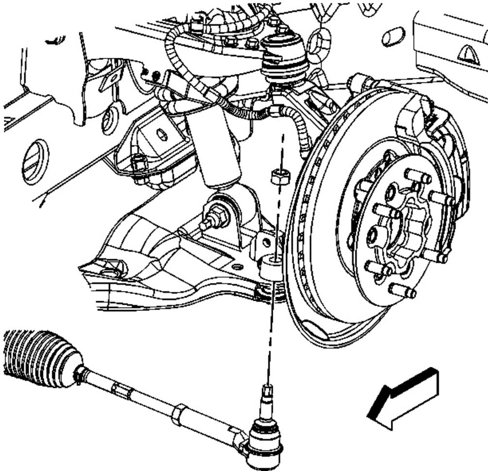
**Fig. 18: View Of Outer Tie Rod Retaining Nut**
