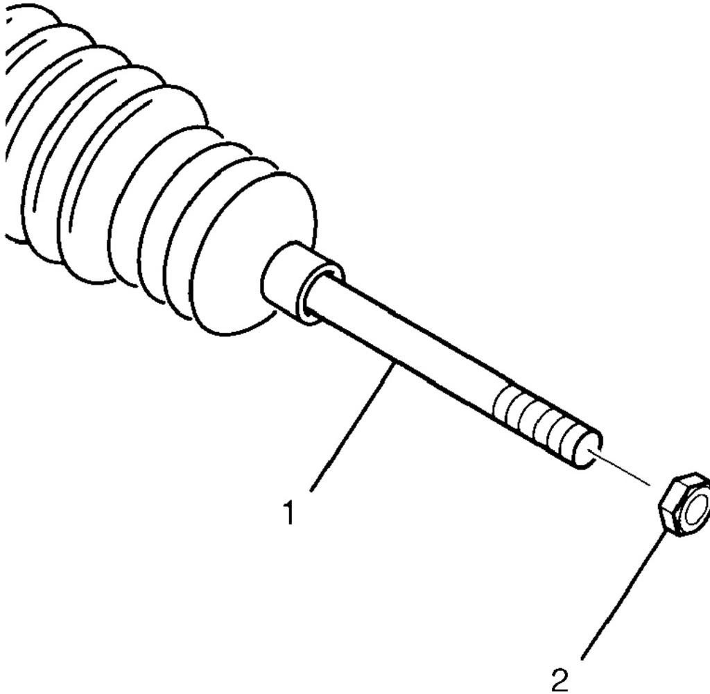
**Fig. 30: View Of Inner Tie Rod & Hex Jam Nut**
