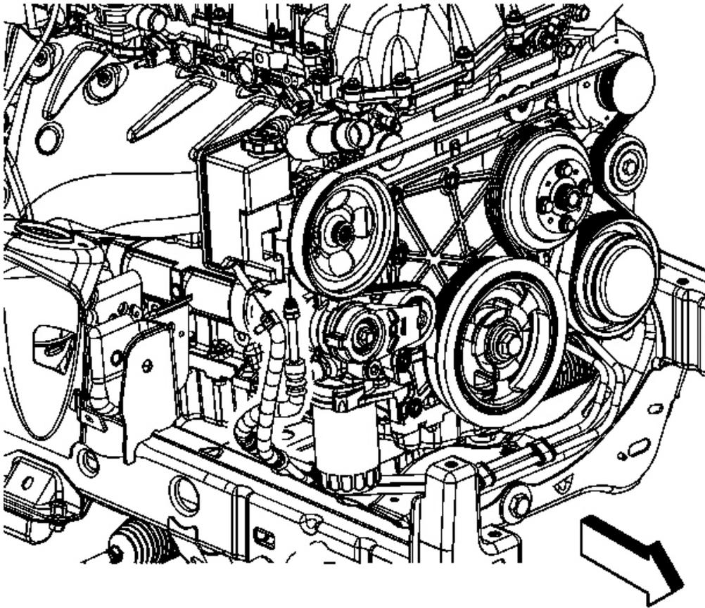
**Fig. 31: View Of Power Steering Pressure Hoses**
