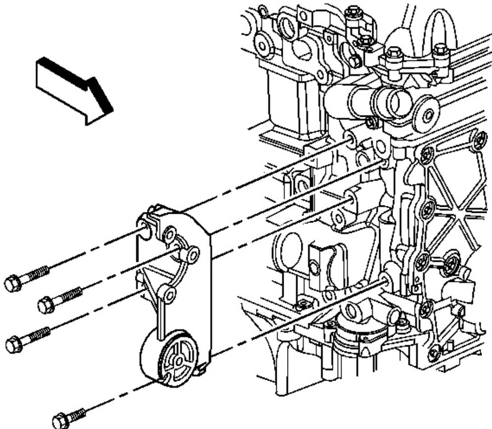
**Fig. 14: Removing/Installing Power Steering Pump Bracket**
