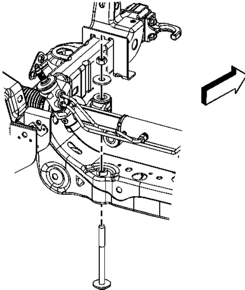
**Fig. 39: View Of Steering Gear Vertical Mounting Bolts**
