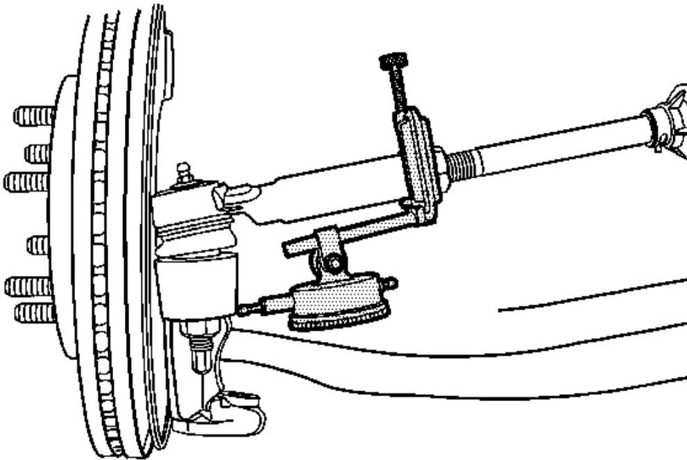
**Fig. 3: Checking Tie Rod-To-Steering Knuckle Lash**
