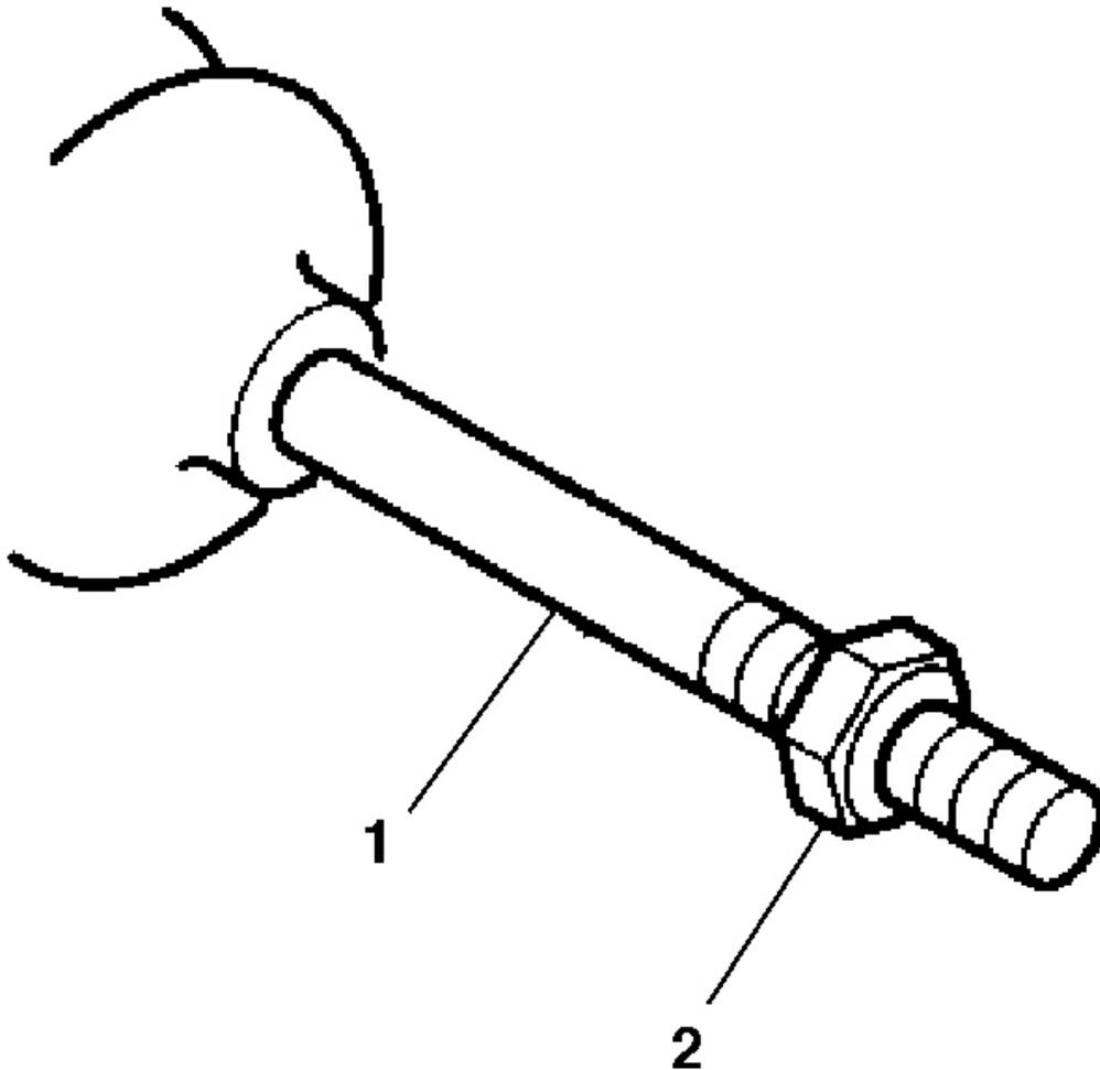
**Fig. 23: Identifying Inner Tie Rod Assembly Jam Nut**
