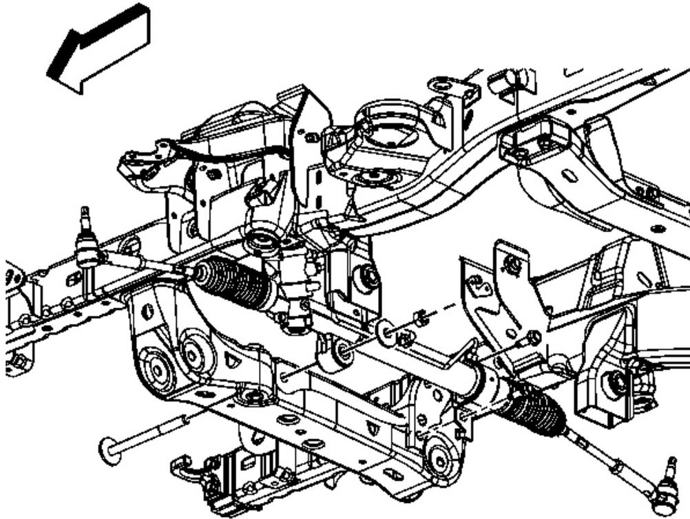
**Fig. 38: View Of Steering Gear Horizontal Mounting Bolts**
