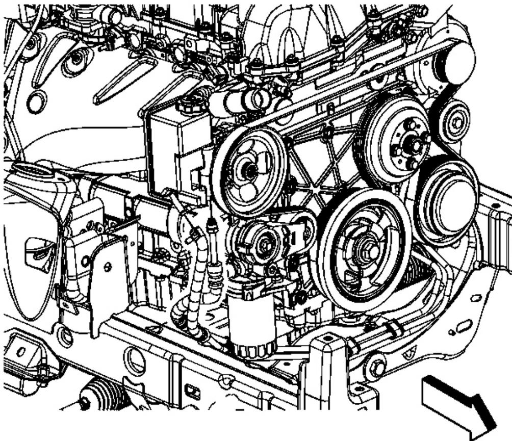
**Fig. 34: View Of Power Steering Pressure Hoses**
