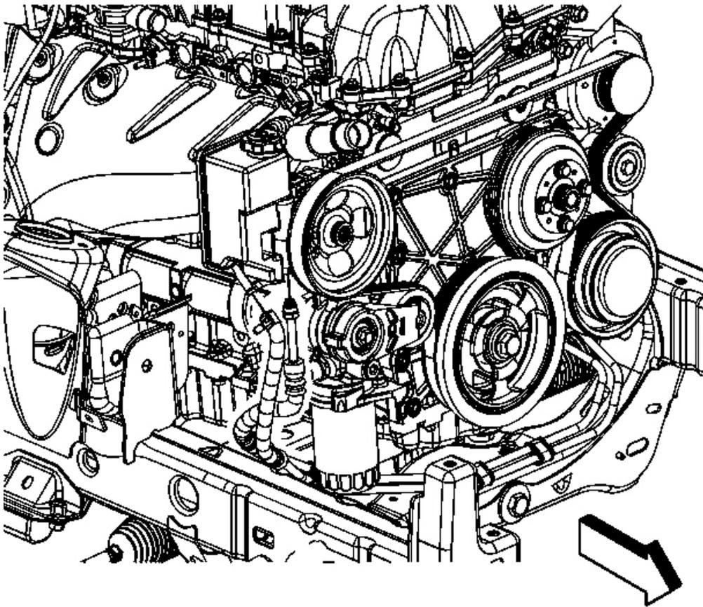
**Fig. 10: View Of Power Steering Pressure Hoses**
