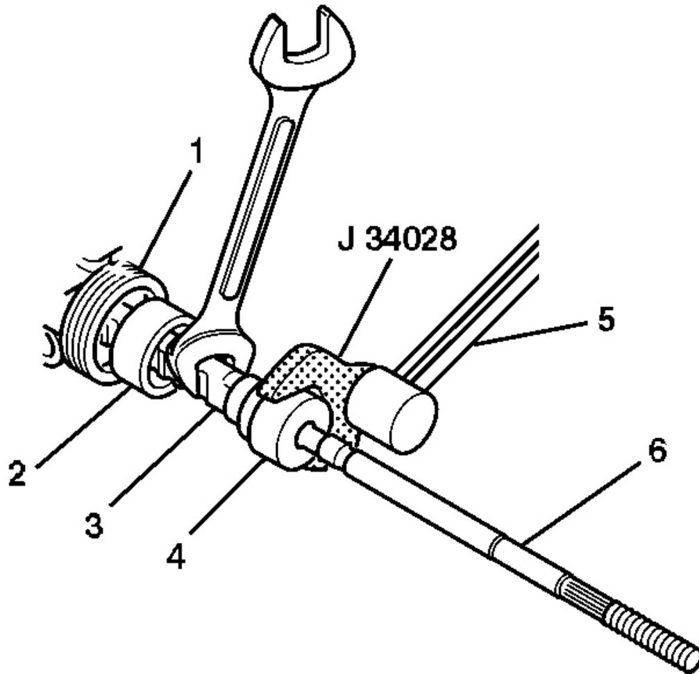
**Fig. 21: Tightening The Inner Tie Rod**
