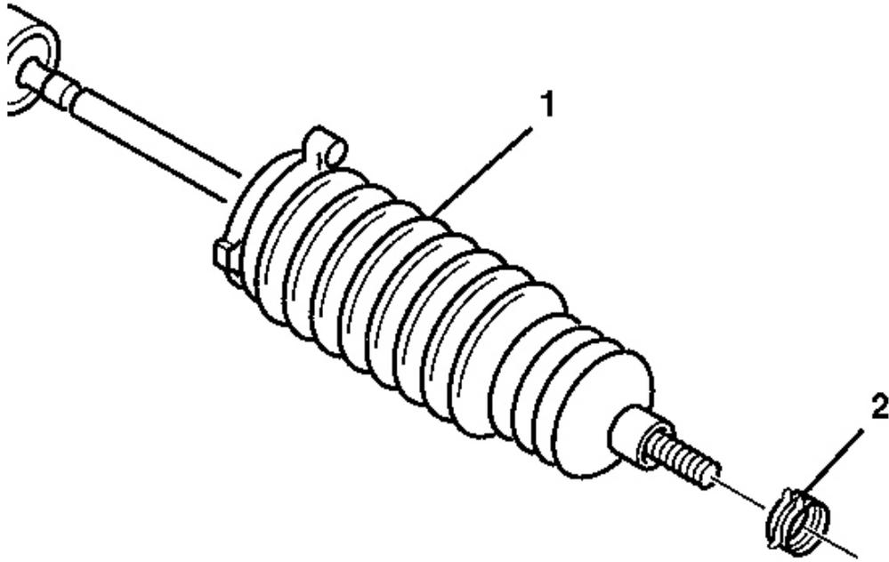
**Fig. 24: View Of Tie Rod End Clamp At Rack & Pinion Boot**
