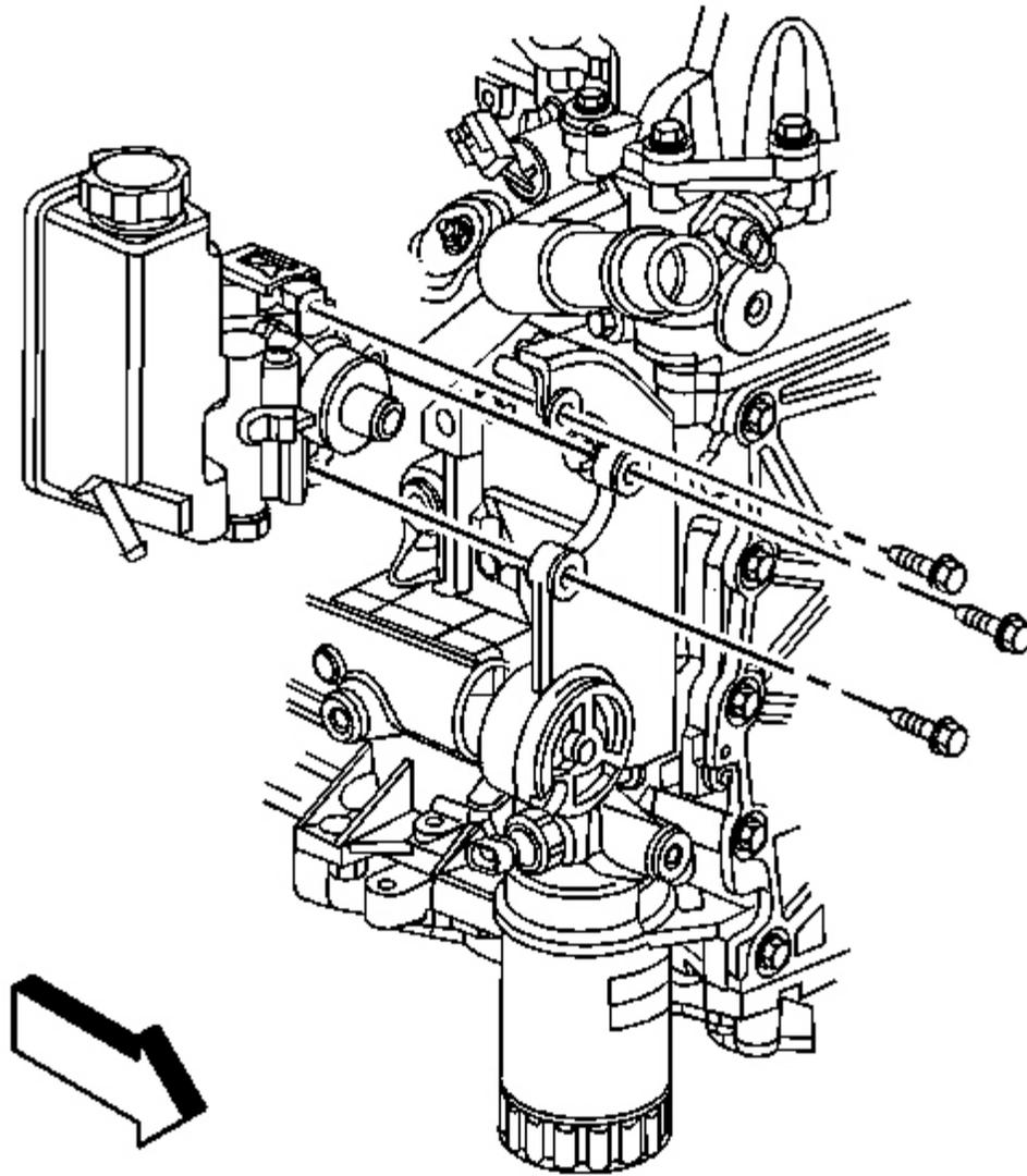
**Fig. 11: View Of Power Steering Pump & Mounting Bolts**
