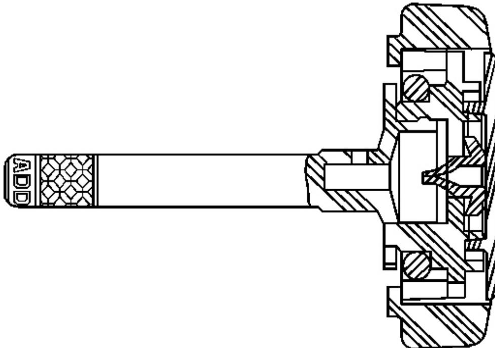
**Fig. 4: View Of Pump Reservoir Cap**
