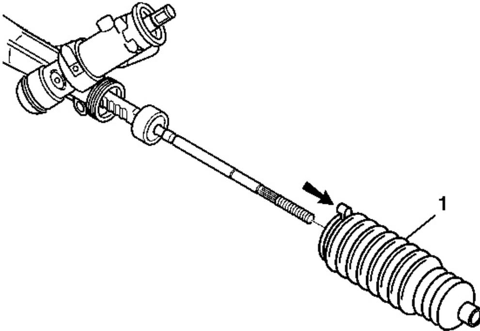
**Fig. 26: Identifying Rack & Pinion Boot & Breather Tube**
