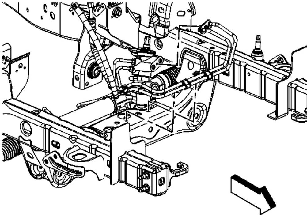
**Fig. 40: View Of Power Steering Hose Assembly**
