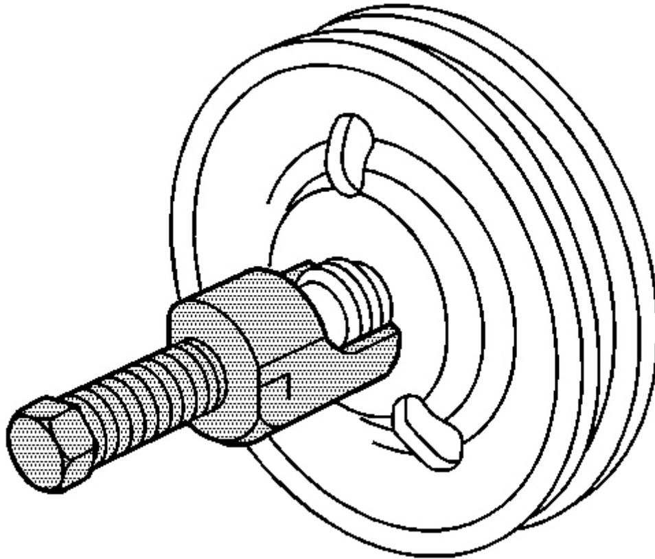
**Fig. 5: View Of Power Steering Pump Pulley Remover**
