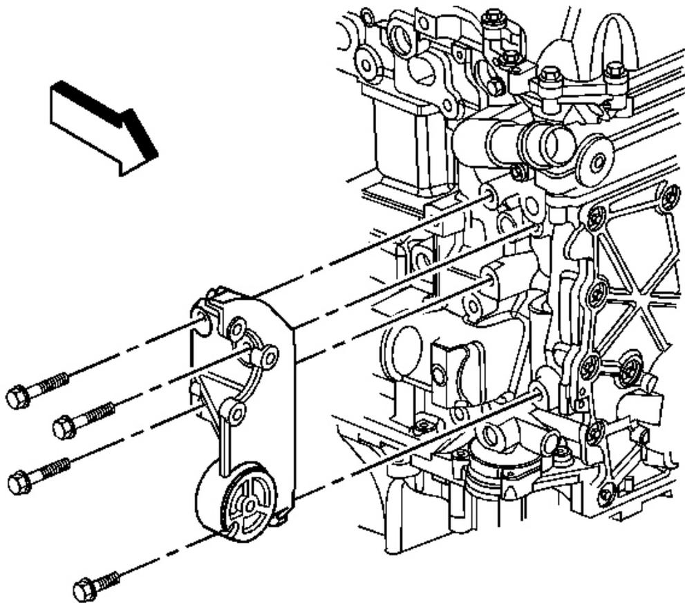
**Fig. 15: Removing/Installing Power Steering Pump Bracket**
