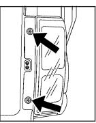
2. Remove the two screws from the taillamp assembly.
