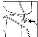
Pull the head restraint up to raise it. To lower the head restraint, press the button, located on the top of the seatback, and push the head restraint down.
