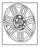
Use the wheel wrench to tighten the nuts firmly. Try to move the tire back and forth slightly to be sure it is secure.
