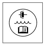
The hydraulic clutch fluid reservoir cap has this symbol on it. See Engine Compartment Overview on page 322 for reservoir location.
