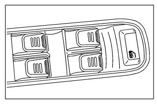
The power window controls are located on the armrest of each door.
