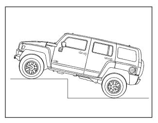
Your vehicle can climb a 16 inch (40.6 cm) vertical step. Step climbing is best done by approaching the step at an angle rather than straight on.
