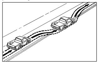
If the level of the shoulder is only slightly below the pavement, recovery should be fairly easy. Ease off the accelerator and then, if there is nothing in the way, steer so that your vehicle straddles the edge of the pavement. You can turn the steering wheel up to one-quarter turn until the right front tire contacts the pavement edge. Then turn your steering wheel to go straight down the roadway.
