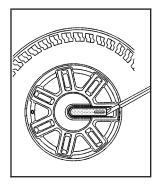
2. Remove the center cap, if equipped, by placing the flat end of the wheel wrench in the slot on the wheel and gently pry the center cap out.
