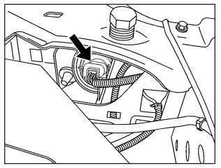
3. Turn the bulb socket counterclockwise to remove it from the headlamp assembly and pull it straight out.
