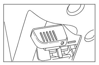
The tilt lever is located on the left side of the steering column, under the turn signal lever.
