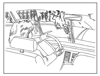
As you brake, your computer keeps receiving updates on wheel speed and controls braking pressure accordingly. Remember: ABS does not change the time you need to get your foot up to the brake pedal or always decrease stopping distance. If you get too close to the vehicle in front of you, you will not have time to apply your brakes if that vehicle suddenly slows or stops. Always leave enough room up ahead to stop, even though you have ABS.
