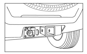
Connect the adapter with the tab pointing up. The flip cap on the vehicle's seven-wire harness will lock onto the tab (see arrow in the previous graphic) and help hold the adapter in place. Plug the four-way pin connector onto the adapter.
