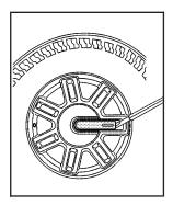
1. Remove the center cap by placing the flat end of the wheel wrench in the slot on the wheel and gently pry the center cap out.
