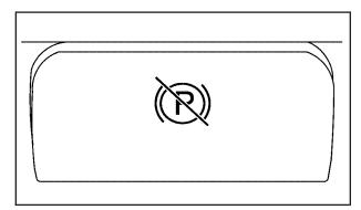
To release the parking brake, hold the regular brake pedal down. Pull the bottom edge of the lever, located above the parking brake pedal, with the parking brake symbol, directly rearward to release the parking brake.
