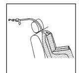
If the position you are using has a fixed head restraint and you are using a single tether, route the tether over the head restraint.
