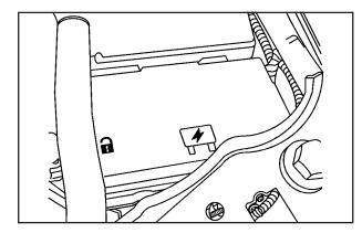
The engine compartment fuse block is located on the driver's side of the engine compartment. See *Engine Compartment Overview on page 322* for more information on location.
