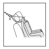
If the position you are using has a fixed head restraint and you are using a dual tether, route the tether around the head restraint.
