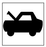
1. Pull the handle with this symbol on it. It is located inside the vehicle on the lower left side of the instrument panel.
