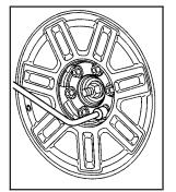
Turn the wheel wrench counterclockwise to loosen the wheel nuts. Do not remove them yet.
