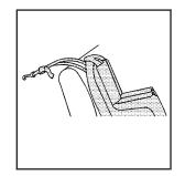
If the position you are using does not have a head restraint and you are using a dual tether, route the tether over the seatback.
