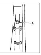
To move it down, press the release button (A) and move the height adjuster to the desired position. You can move the height adjuster up just by pushing up on the shoulder belt guide.
