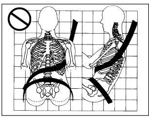
A: The shoulder belt is worn under the arm. It should be worn over the shoulder at all times.
