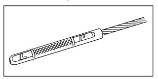
If the oil is below the cross-hatched area (L), you will need to add at least one quart/liter of oil. But you must use the right kind. This section explains what kind of oil to use. For engine oil crankcase capacity, see *Capacities and Specifications on page 422*.
