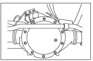
To get an accurate reading, the vehicle should be on a level surface. The proper level is from 0 to 3/8 inch (0 mm to 10 mm) below the bottom of the filler plug hole, located on the rear axle.
