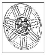
3. Use the wheel wrench to remove the wheel nuts securing the spare tire.
