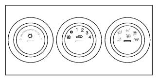
This system controls the heating, cooling, and ventilation of the vehicle. In-between modes are available by moving the right control knob between modes with symbols. The in-between mode will be a combination of the two modes that the control is centered between.
