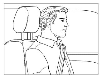
Adjust the head restraint so that the top of the restraint is at the same height as the occupant's head. This position reduces the chance of a neck injury in a crash.
