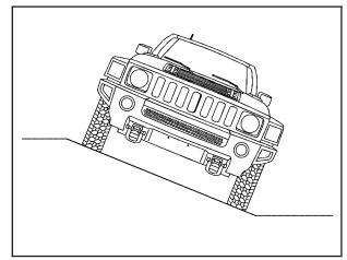
Also, your vehicle should be able to traverse a 40% (22 degrees) side slope at 6 mph (9.7 km/h) while fully loaded on high friction surfaces.
