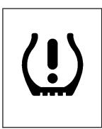
As an added safety feature, your vehicle has been equipped with a tire pressure monitoring system (TPMS) that illuminates a low tire pressure telltale when one or more of your tires is significantly under-inflated.
