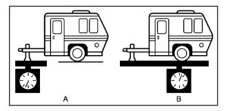
The trailer tongue weight (A) should be 10 percent to 15 percent of the total loaded trailer weight (B), up to a maximum of 500 lbs (227 kg) with a weight carrying hitch or a weight distributing hitch.
