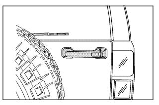
To open the swing-gate, pull the door handle. Pull the swing-gate rearward slightly and it will automatically open.
