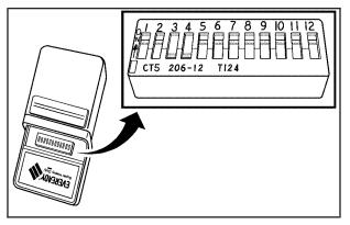
If you do not know if your garage door opener is a fixed code or rolling code device, open your garage door opener's remote control battery cover.
