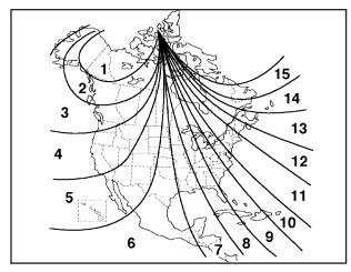
3. Press the compass/temperature button on the bottom of the mirror until the new zone number appears in the display. After you stop pressing the button, the display will show a compass direction within a few seconds.
