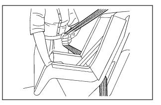
5. Pull the rest of the shoulder belt all the way out of the retractor to set the lock.
