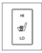
If your vehicle has this feature, the controls are located on the outboard side of the front seats.
