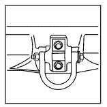
Your vehicle has two recovery loops at the front of the vehicle and one at the rear of the vehicle.
