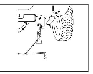
**Rear Tire Flat:** You will need to use the jack handle and both jack handle extensions. Attach the wheel wrench to the jack extensions. Attach the jack handle to the jack. From the rear of the vehicle align the jack under the rear axle. Turn the wheel wrench clockwise to raise the vehicle. Raise the vehicle far enough off the ground so there is enough room for the spare tire to clear the ground. 5. Turn the wheel wrench clockwise to raise the jack head to the lifting point.
