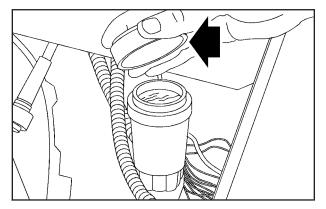
It is not necessary to regularly check clutch fluid unless you suspect there is a leak in the system. Adding fluid will not correct a leak.
