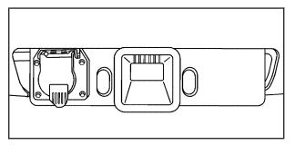
If your vehicle is equipped with a trailer towing package, the rear bumper harness will have a seven-pin universal heavy-duty trailer connector attached to a bracket on the hitch platform. The trailer towing harness contains the following seven trailer circuits:
