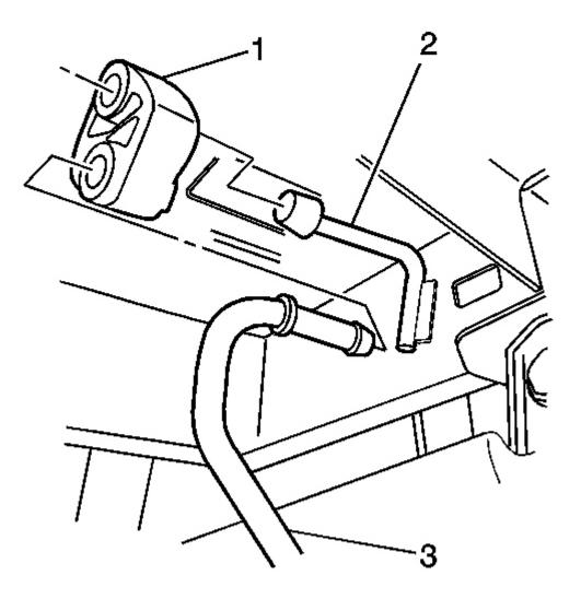
**Fig. 21: View Of Exhaust Pipe Hanger** Courtesy of GENERAL MOTORS CORP.
