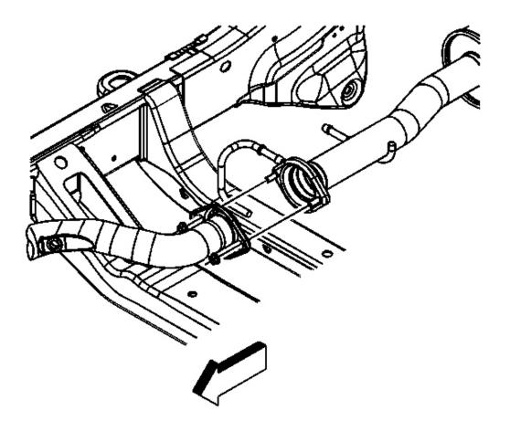
**Fig. 30: View Of Nuts Securing Muffler To Catalytic Converter Courtesy of GENERAL MOTORS CORP.**  2007 ENGINE Engine Exhaust - H3
